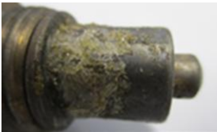
Figure 11. soot/ash on the sensor head
