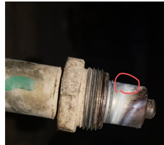
Figure 12. Urea on the sensor head
