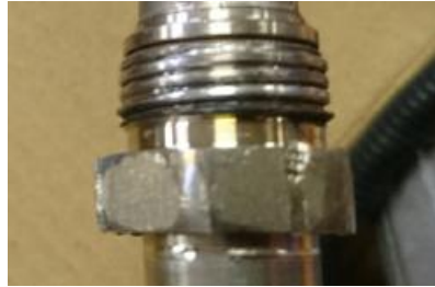
Figure 10. Damaged sensor thread and nut
